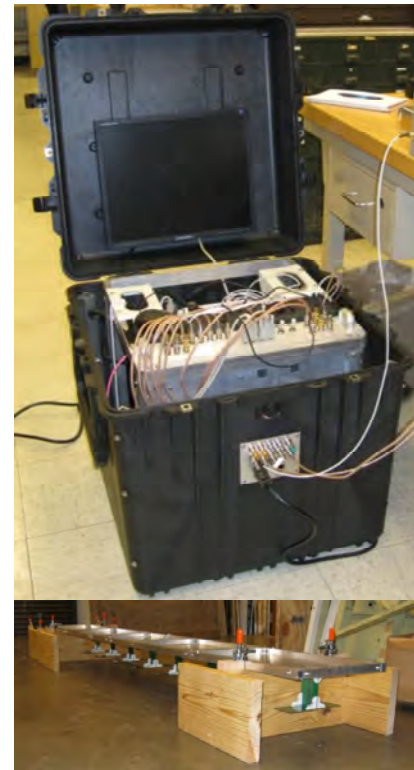
Figure 50: Photo on left is the surface-based Accumulation Radar System inside the pelican case. Photo on right is the assembled antenna array and mounting structure. (Photos courtesy of Judith Riley).
