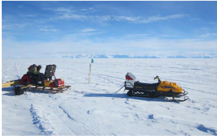
Figure 52: Photo of Peter Burkett working with the surface-based Accumulation Radar on the Ross Ice Shelf, with Transantarctic Mountains in the background. The radar antennas (in box at rear of sled) and the antenna hardware (in black case on sled) were transported by Twin Otter aircraft and towed by skidoo. (Photo courtesy of Sridhar Anandakrishnan)
