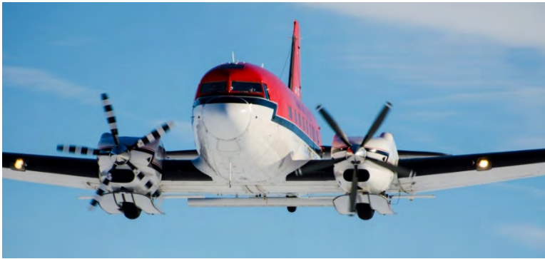
Figure 45: Photo of MKB Basler in flight with CRISIS radar and antenna configuration. The fuselage-mounted antenna array for the UWB UHF/VHF Radar System can be seen mounted to the fuselage just aft of the wings. (Photo courtesy of Alec Bowman).
