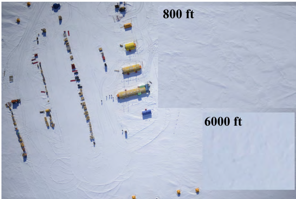
Figure 37: Image of camp from 800 ft AGL with two insets showing snow detail from 800 ft and 6000 ft. Snow features are very crisp in 800 ft imagery and appear blurred, but still visible, in 6000 ft imagery.
