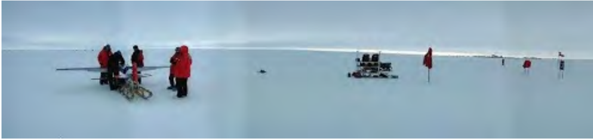
Figure 48: Photo of radar ground test setup. See G1X UAS (with radar inside) attached to sled on left, with UAS ground control station in center/right of photograph. (Photo courtesy of Alec Bowman).
