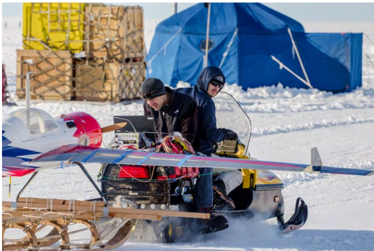
Figure 47: Photo of ground test of dual-frequency radar installed inside G1X UAS with antennas integrated in wings. The UAS was attached to a sled and towed behind a snowmobile to measure the runway’s ice thickness. In this photo, Carl Leuschen is conducting the radar test and Nicholas Brown is driving the snowmobile. (Photo courtesy of Alec Bowman).
