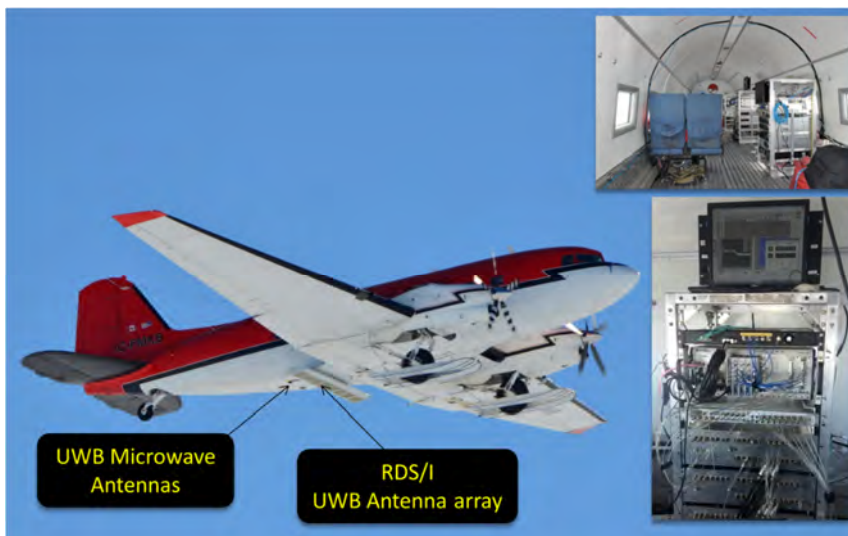
Figure 3: Photograph of the BT-67 platform equipped with antenna array for the UWB radar depth sounder/imager and microwave antennas for the Ku-band/Snow radars. The top inset shows a photograph of the cabin equipped with the instrument package. The bottom inset shows a photograph of the rack containing UWB radar depth sounder electronics.
