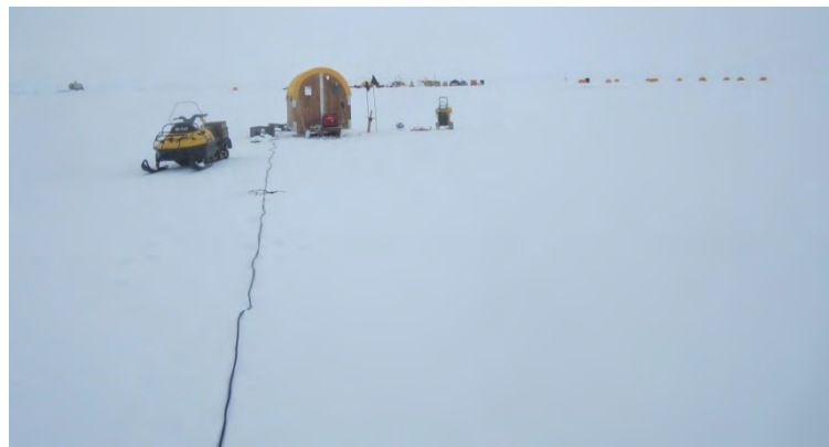
Figure 53: Photo of seismic testing at SLW/CReSIS camp. The shelter contains the seismic recording equipment, and the cable in the foreground connects to buried geophones. (Photo courtesy of Sridhar Anandakrishnan)
